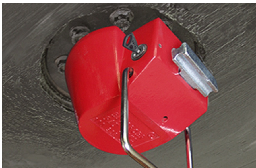
Figure 14.4 King pin lock.
